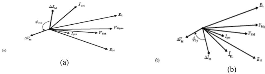
Fig.6 Phasor diagram for Algorithm-3
